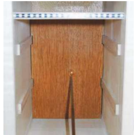
▲ Pic 22 The secret drawer is retrieved using a magnet on a stick
